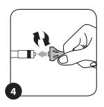
Pump no more than 6 times. This will pressurize the unit to approximately 35 psi. Take note of the force required on the last pump and use this as a guide for when to stop pumping on future charges so that you do not over-pressurize the unit.
