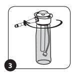
Grasp the OtoClear Tip and twist onto the luer lock fitting of the adapter until it stops.
